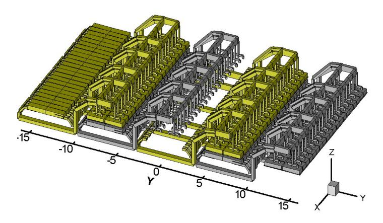
Example of busbars geometry construction (6 risers, side by side cells)
