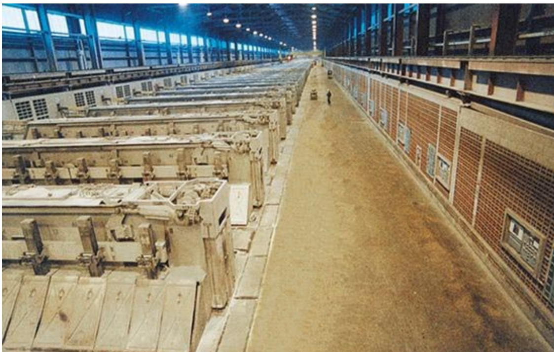
Figure 2: Modern smelter “potroom” building configuration
