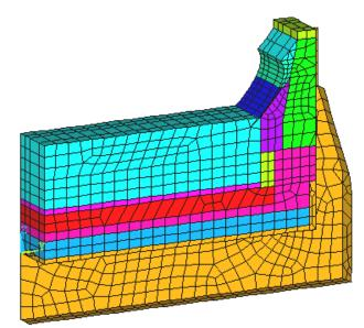
Figure 2: Cathode side slice model mesh
