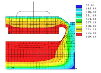
Figure no 8: 2D full cell slice model isotherms
