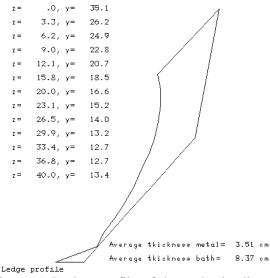
Figure 5: Ledge profile of the cathode slice model
