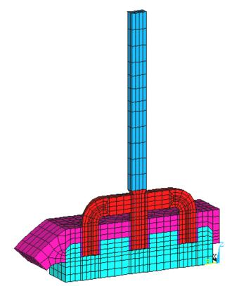
Figure 1: Half anode model mesh
