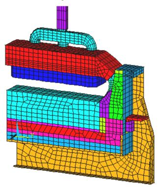
Figure 3: 3D full cell slice model mesh
