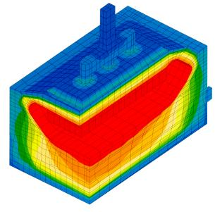
Figure 7: VAW's full cell corner model isotherms[12]
